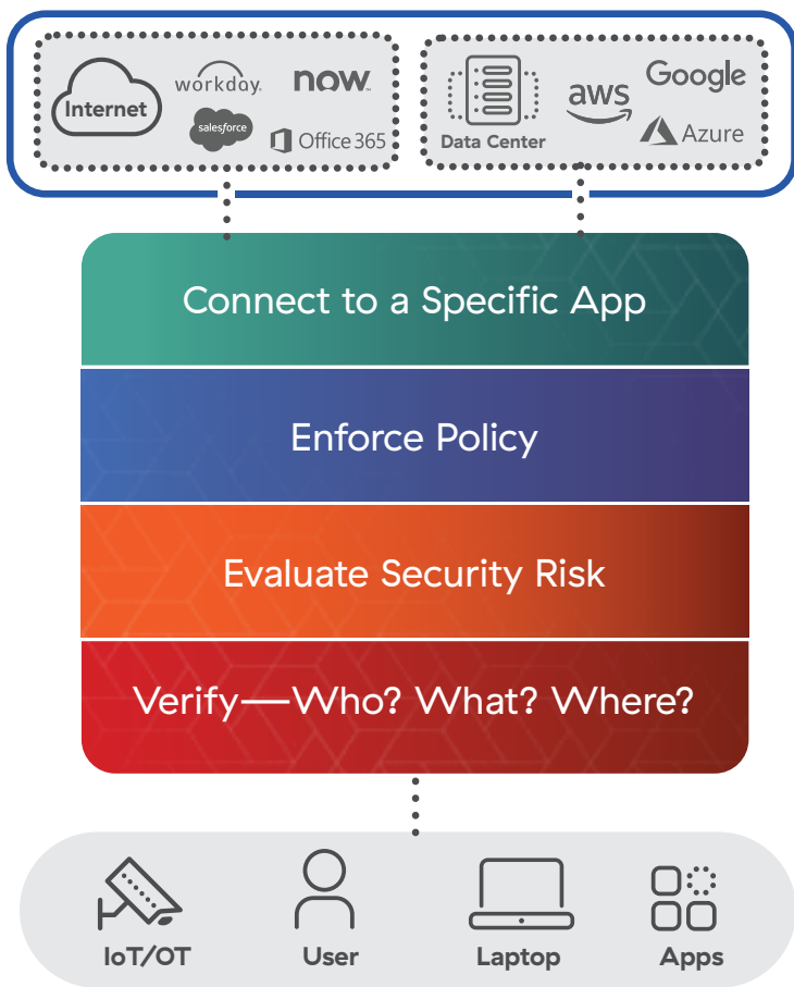
Figure 20: Steps that a zero trust architecture (ZTA) takes before connecting a user to reduce the risk of a cyber breach.
